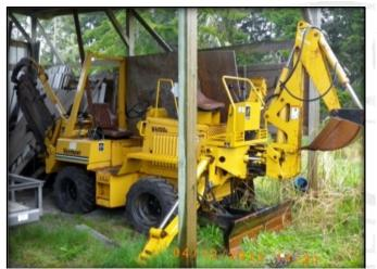
The District acquired a 1993 Vermeer V-4150A tractor outfitted with a Vermeer V-1650 Trencher and a Vermeer B500/600 Backhoe along with the purchase of Ocean Park Water Company. The Tractor has 533 hours of use recorded on its hour meter. The Vermeer tractor became obsolete when the District acquired the Kamatsu Backhoe in 2006. The condition of the tractor is
