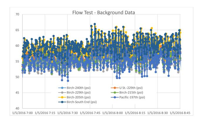
In this case, the South Pump Station was turned on at about 7:45 AM. Both flow tests were conducted after 9:00 in the morning. The South Pump Station was in service for both tests. The flow tests were conducted with very little background water demand present within the system, which generally allows for more consistent model calibration. A pitot gauge and diffuser were
